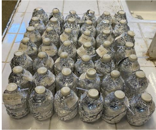
Figure 3.7. The reactor filled with inoculum and cattle manure wrapped with aluminum foil in Set 1
