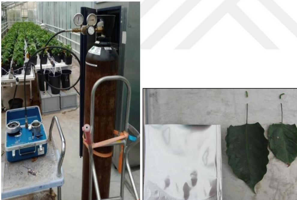
Figure 3.5. Pictures of the scholander bomb and the leaf retrieval method in an aluminum foil.
