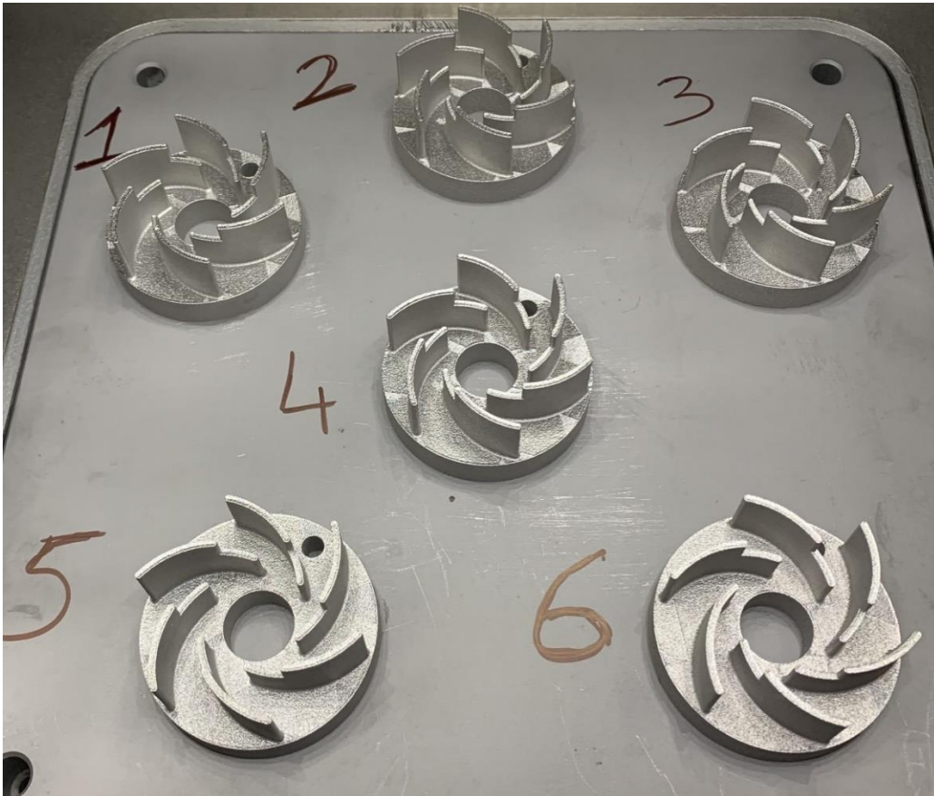
Figure 29: Manufactured impellers for distortion measurement
