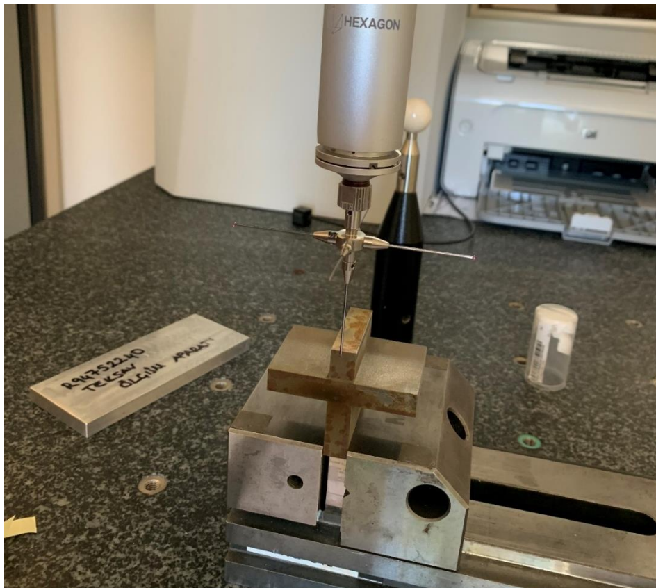
Figure 35: Measurement of Surface Deformations
