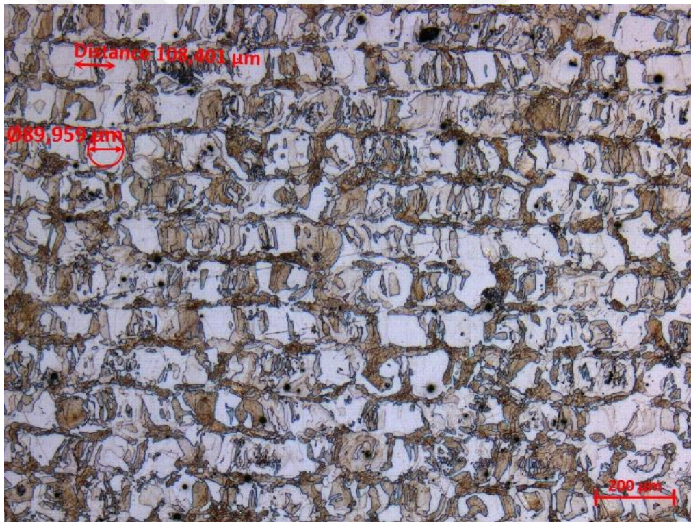
Figure 42: Optical microscopy of as built 17-4 PH SS in the build direction
