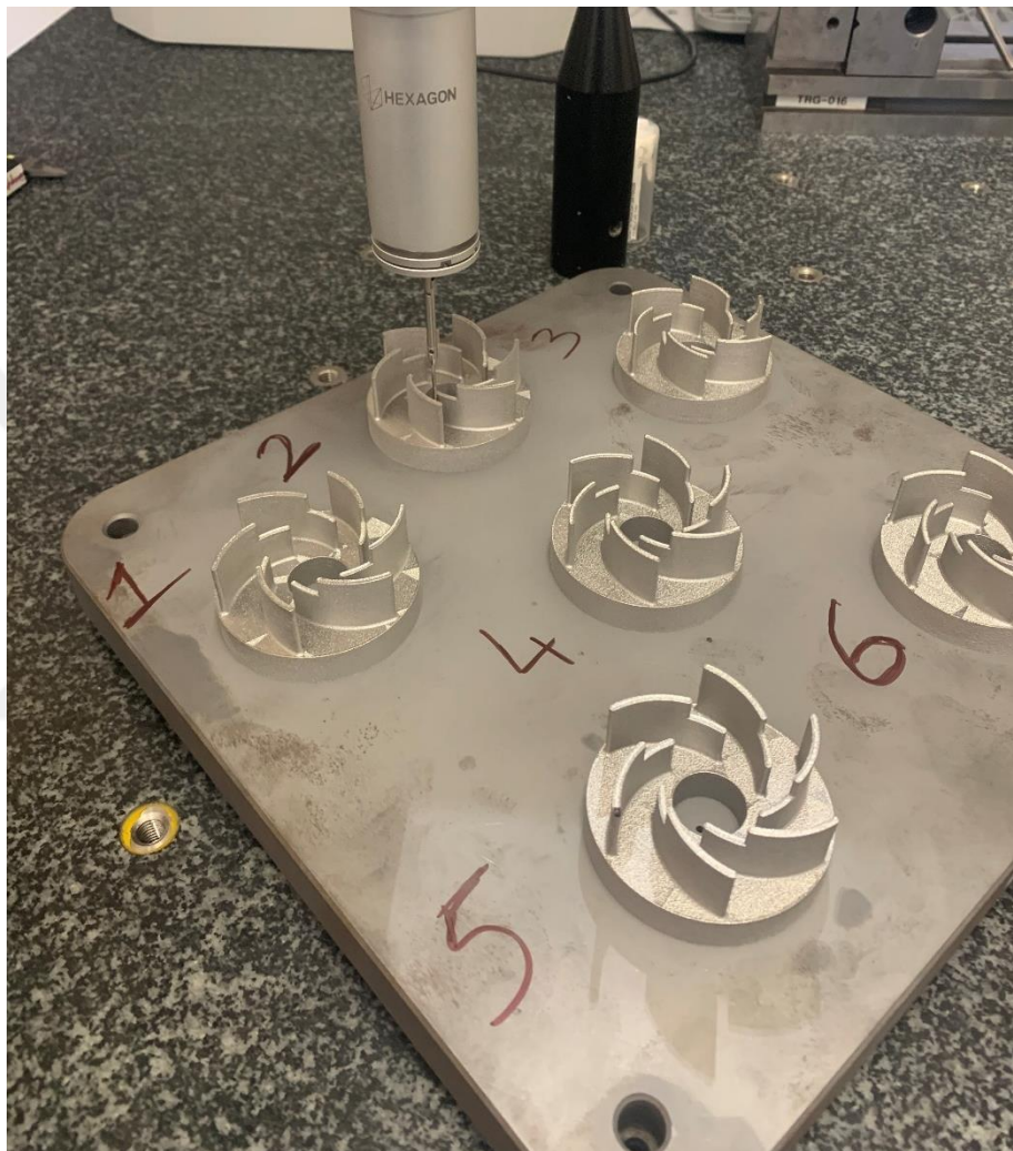
Figure 30: CMM dimensional measurement of impellers
