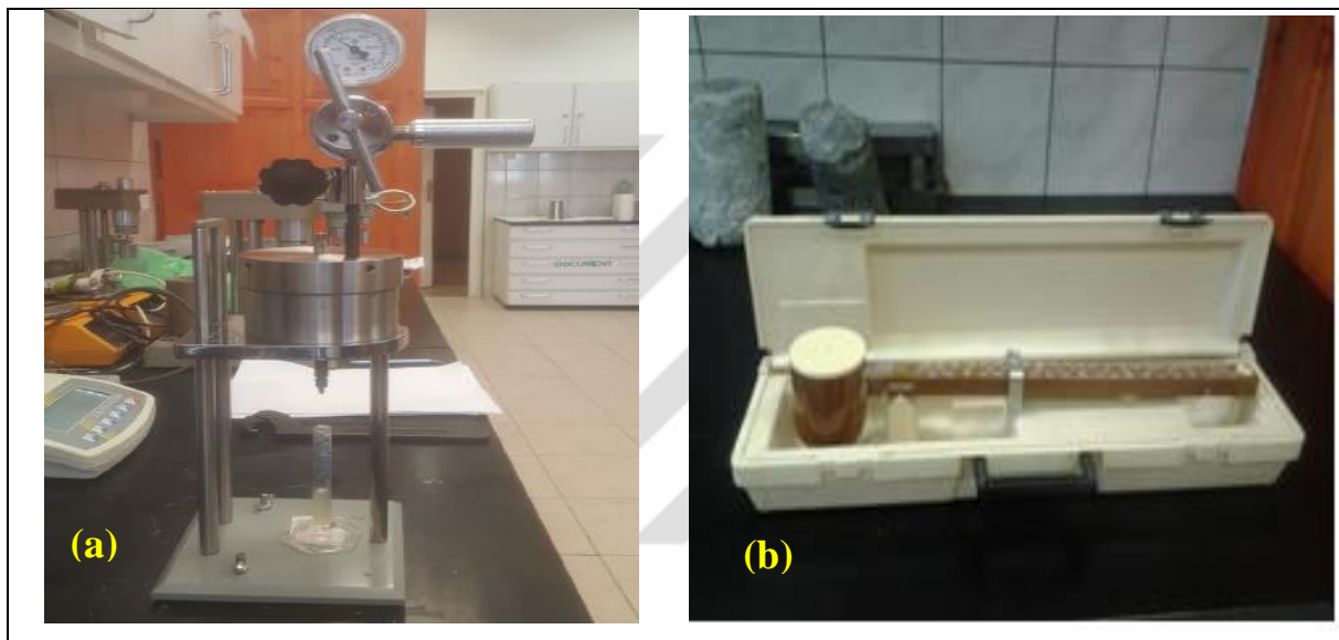
Figure 6.17. Differential sticking tester (a), mud balance (b).
