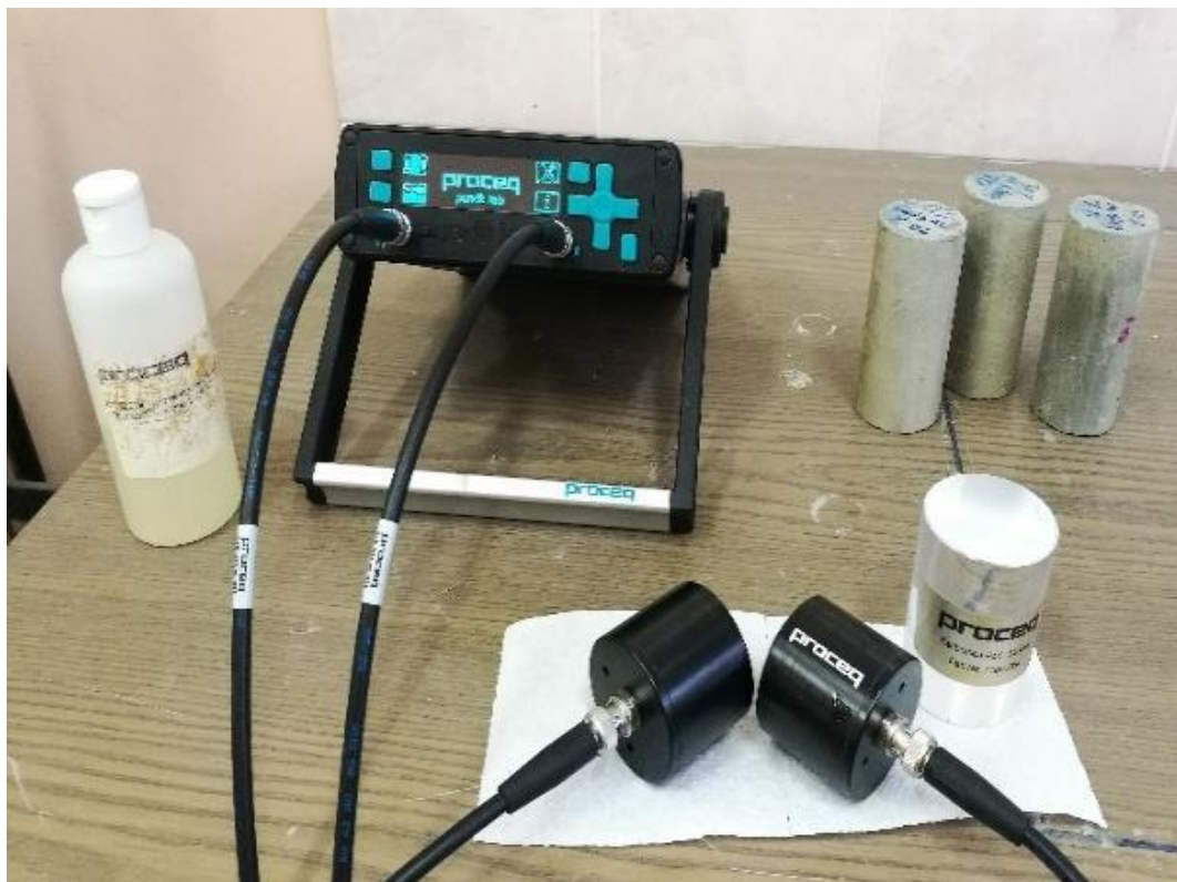
Figure 3.14 Ultrasonic pulse velocity test instrument.
