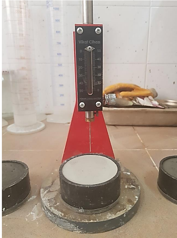
Figure 3.11 Vicat Apparatus Test.
