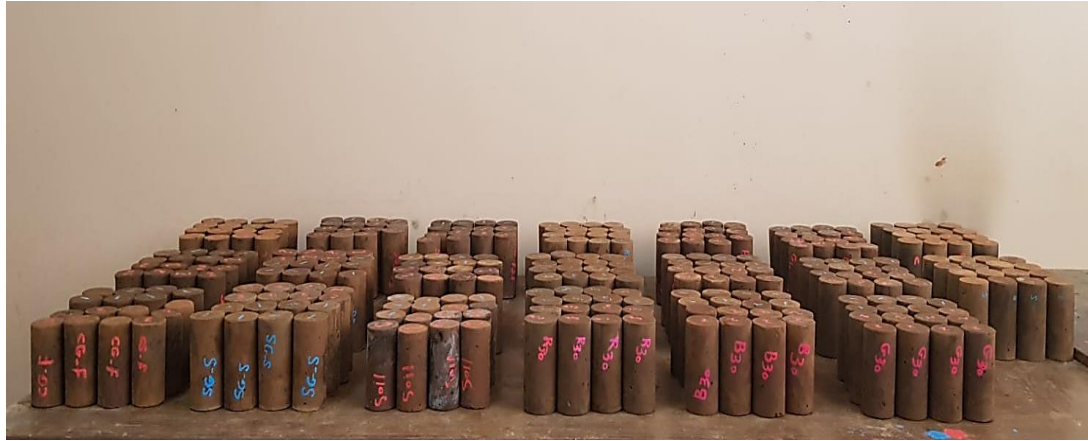
Figure 3.6 Geopolymer-stabilized soil samples.
