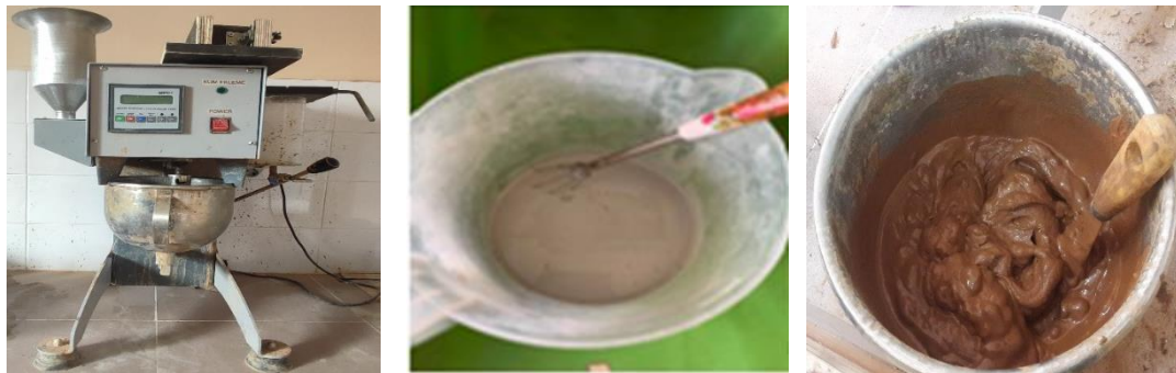
Figure 3.5 Mixing procedure to preparation DSM specimen.
