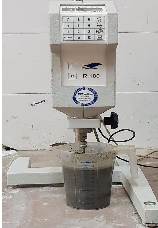
Figure 3.7 Coaxial rotating cylinder Rheometer.
