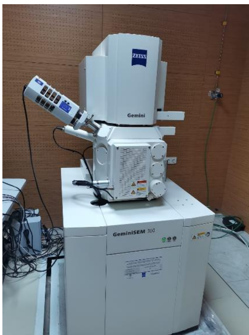
Figure 3.15 SEM device used in this study.
