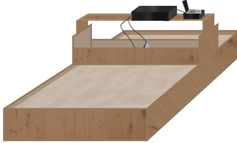
Figure 3.14 Illustration of the GPR configuration utilized for generating experimental training and testing data used by the proposed surrogate-assisted buried object characterization framework
