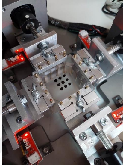
Figure 33: Membrane installed on the stretching device and tested.
