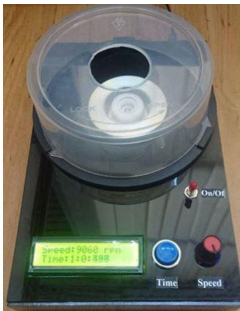
Figure 4: Spin coater device with speed and time controllers (Sadegh-Cheri 2019: 1269).
