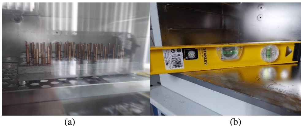
Figure 28: (a) Mold in oven (b) Balancing oven using water gauge.
