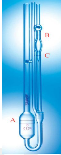
Şekil 1.88 Ubbelohde viskozimetresi Tip 1B-ASTM D 4603'e uygun https://www.cannoninstrument.com/media/assets/product/documents/manual.viscosity.brochure.pdf
