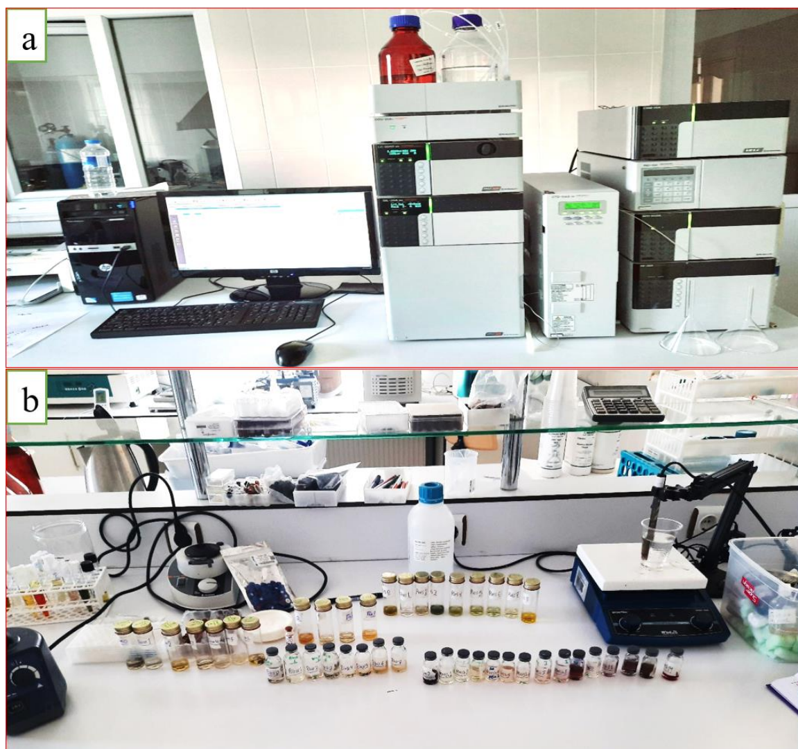
Figure 4.8. (a) Shimadzu HPLC-DAD instrument, (b) Preparation of the sample extracts and fractions for HPLC analysis
