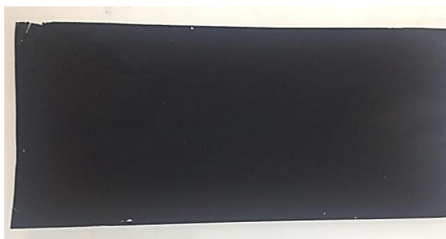
Figure 3.1. Prepared cathode film with C/S = 1.
