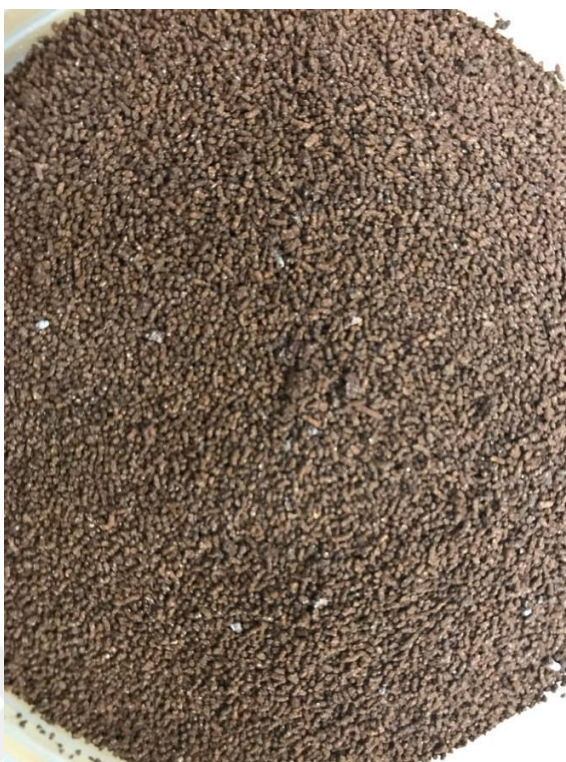
Figure 2.1. Granulated spheres of immobilized glucose isomerase
