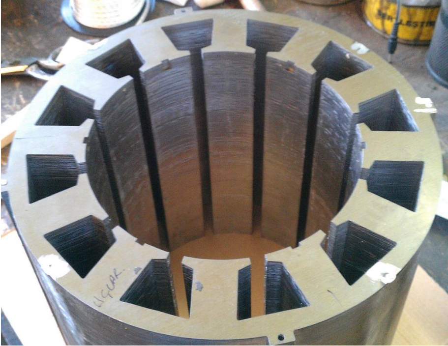
Figure 3.25 : Stator (set ready for winding process).
