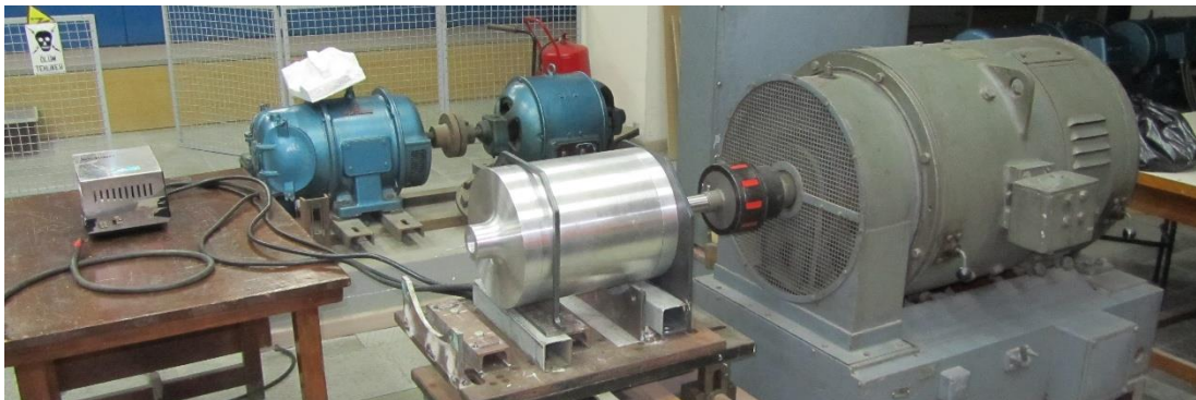
Figure 3.32 : Motor test bench.
