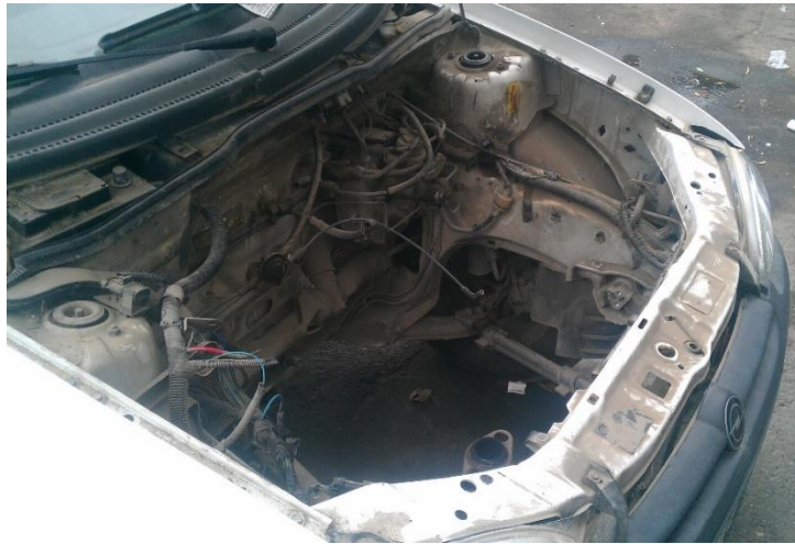
Figure 4.1 : ITU EV after ICE removal.
