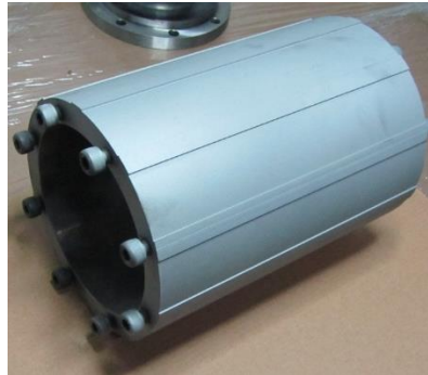
Figure 3.20 : Motor back iron after process.
