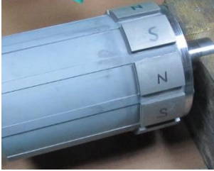
Figure 3.21 : Magnet attachment process.
