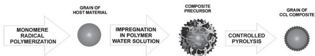
Figure 4.1: CCL covering process of \text{LiFePO}_4 nanoparticles [93].
