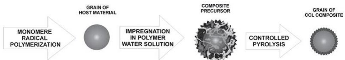
Figure 2.12: Producing CCL covered nanoparticles [93].
