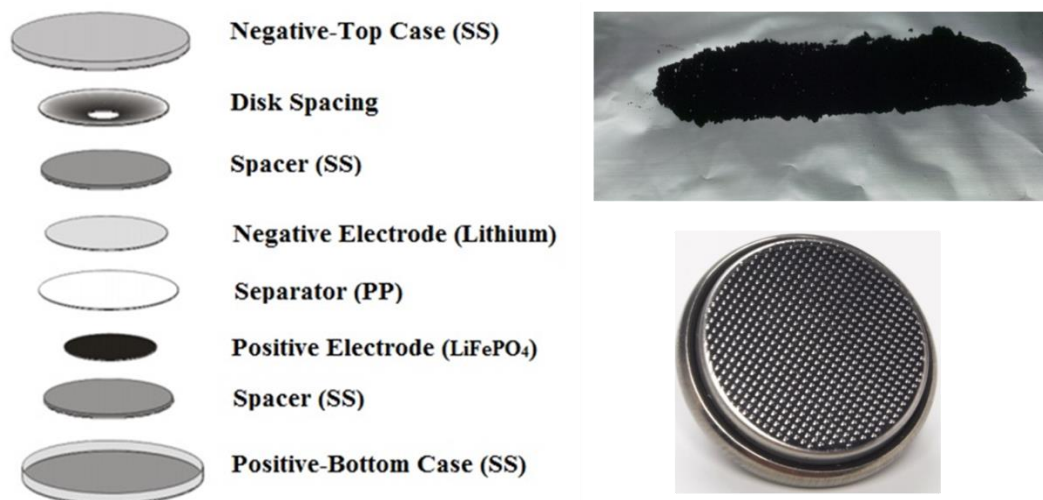
Figure 4.2: An illustration of assembling a coin cell.
