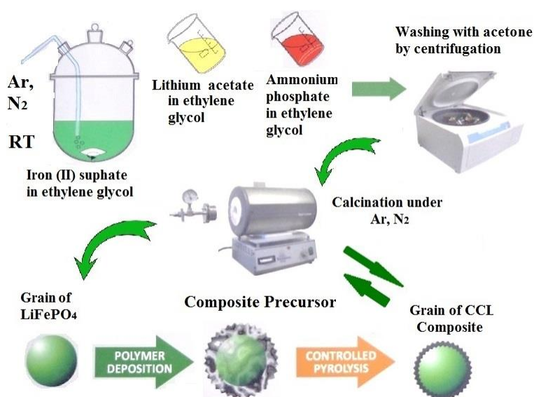
Figure 5.1: Schematic representation of powder production.
