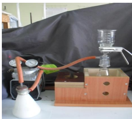
Figure 2.5 Filtration apparatus used for filtration and washing adsorbents (PALL Vacuum Pump filtration flask & funnel)
