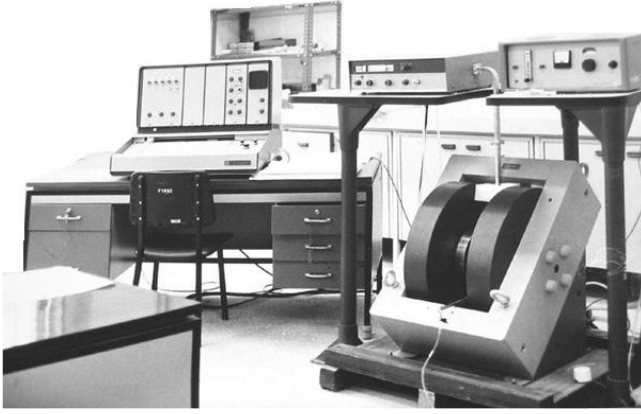
Şekil 3.1: X Band Varian Century Line Series E109 EPR spektrometresi.
