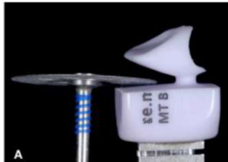
Figure 2.7: Cutting Out Milling Model from CAD/CAM [4].
