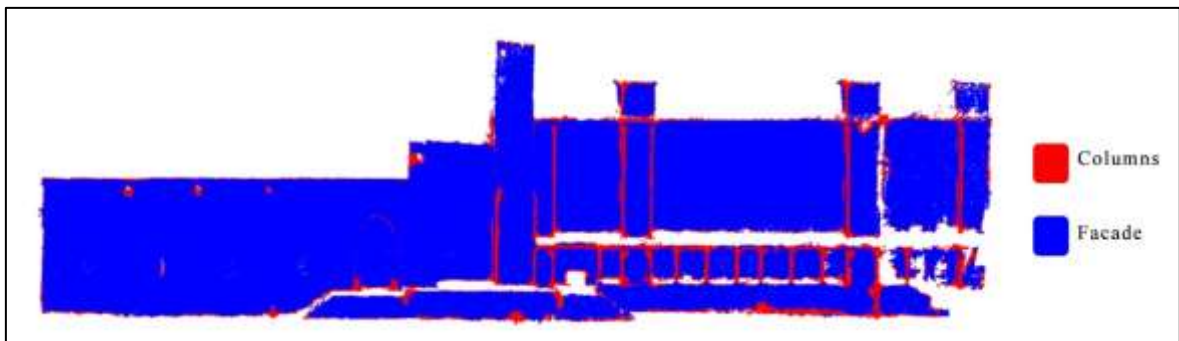
Figure 4.2: Segmentation Result of the Columns' Class from the Trained Dataset on the SW Facade.
