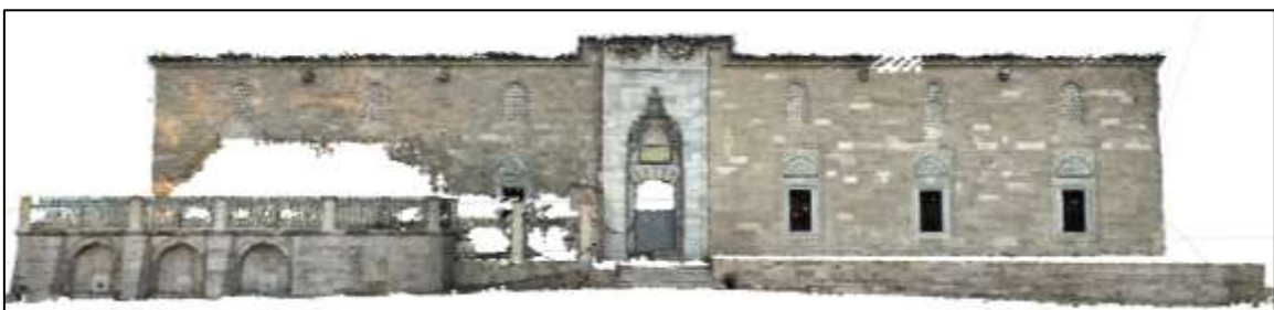
Figure 3.4: A 993,501 Point Cloud Model of the NW Facade, Captured from Agisoft Metashape.
