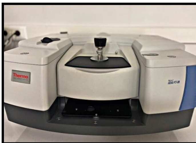
Figure 2.11: Thermo scientific nicoleet iS50 FT-IR used for FT-IR analysis of synthesized GQDs, Fe-MOFs and functionalized hybrid NPs.
