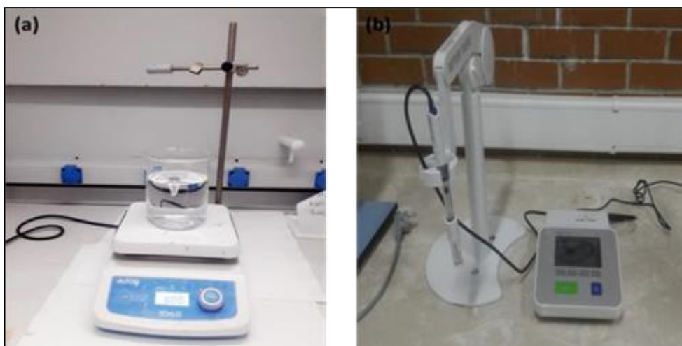
Figure 3.1. (a) magnetic stirrer (b) benchtop pH meter
