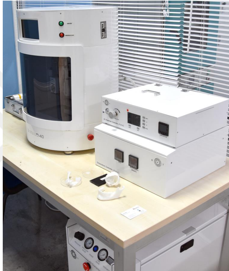
Figure 3.4: Dr. INVIVO 4D2 bioprinter and its auxiliary equipment.
