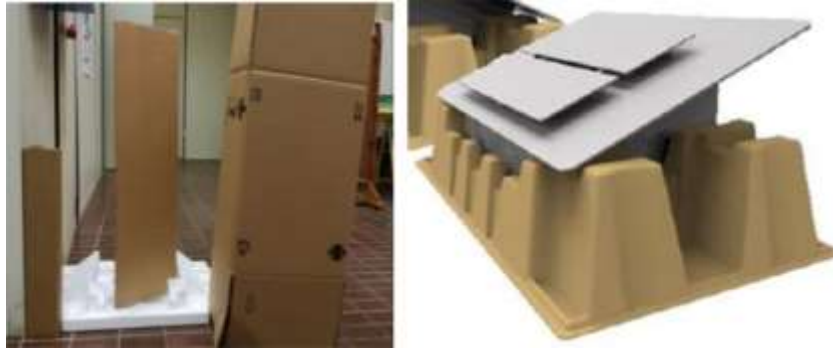
Figure 2.6: Items of the reference packaging for the vertical cooker hood (left) and the prototype of the interior base in the molded pulp (right)
