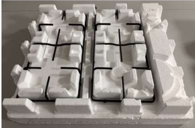
Figure 3.34: EPS model of molded cellulosic top part outer for metal gas hobs.
