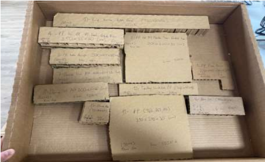
Figure 5.17: Honeycomb panel specimens.
