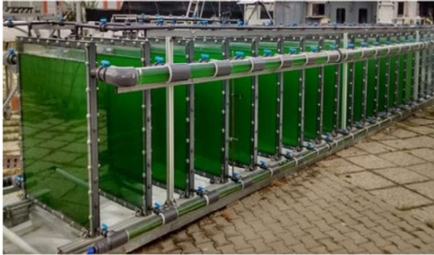
Figure 2.4 : Flat panel photobioreactor setup (Lindblad et al., 2019).
