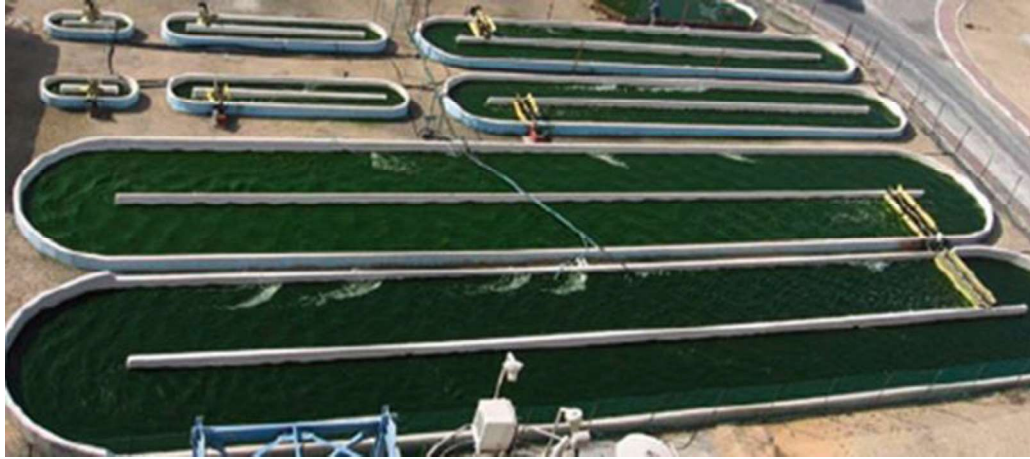
Figure 2.2 : Open raceway ponds with paddle wheels operated in outdoor mode from UK. Different sizes of the ponds for preparing inoculum cultures (Koller, 2015).
