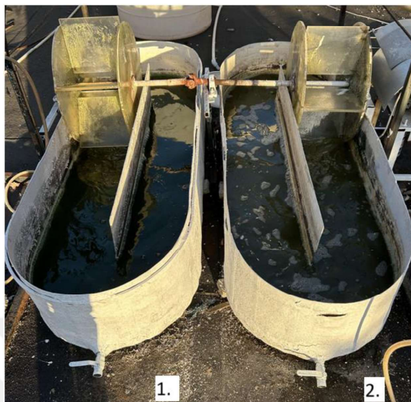
Figure 3.8 : Open Raceway Setup. 1. Coculture media, 2. Monoculture media.
