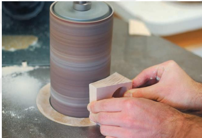
Figure 2.11. Finishing wood on a sanding machine (Halgrimsson, 2012)
