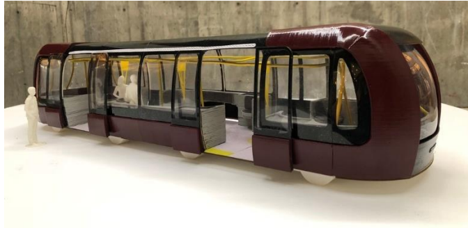
Figure 4.48. T3's bus mockup submission earning a grade of 3 for material quality, and a grade of 2 for component detailing
