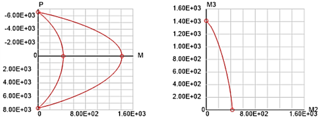
Şekil 3.15 : HE450B kolon PERFORM-3D [17], P-M2-M3 StrengthSectionSteel.
