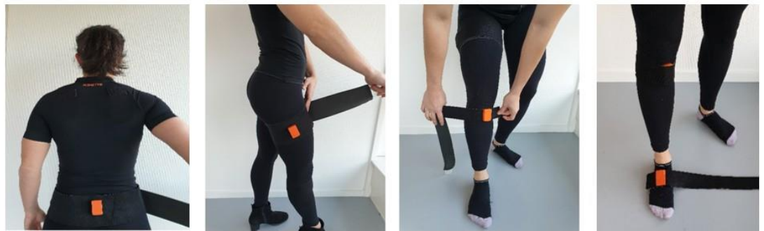
Figure 15. Position of XSENS sensor for the lower body part (Pelvis, Upper Leg, Lower Leg, Foot).
