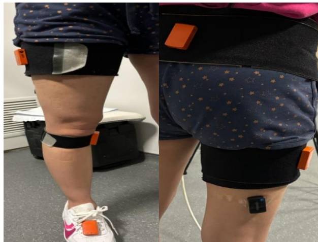
Figure 16. The XSENS sensors on the lower body part were used during the experiment.
