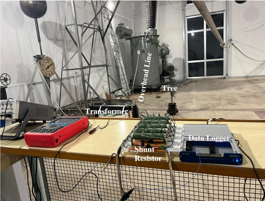
Figure 3.2 : The first test set-up picture for a tree-leaning overhead line in the laboratory environment.
