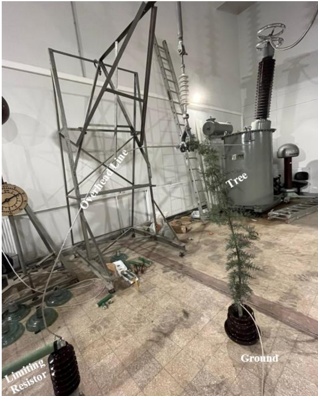
Figure 3.3 : The second test set-up picture for a tree-leaning overhead line in the laboratory environment.
