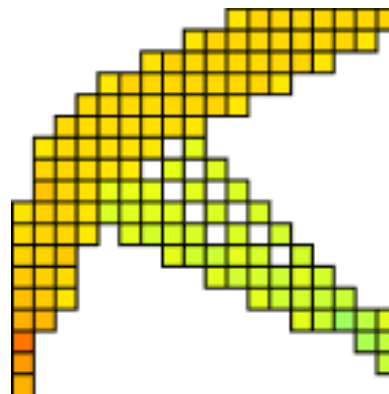
Figure 4.38: Checkerboard pattern in Membrane Model
