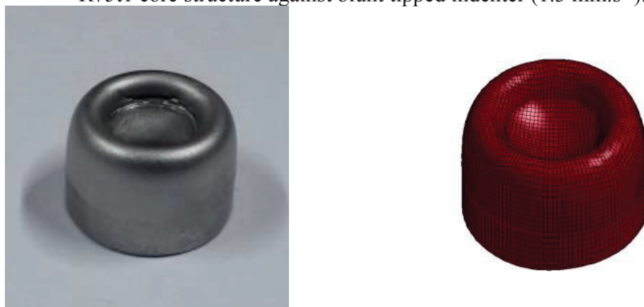
Figure 4.31. Comparison of experimental and numerical deformation of R75t1 core structure against blunt tipped indenter ( 1.3 \text{ mm.s}^{-1} ).
