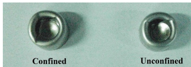
Figure 6.2. Comparison of test results and deformed specimens with confined and unconfined states (R75t1 core units against blunt tipped indenter).
