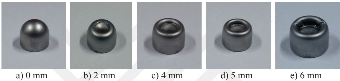
Figure 4.20. Deformation progress of R75t1 specimen against blunt tipped penetrator.
