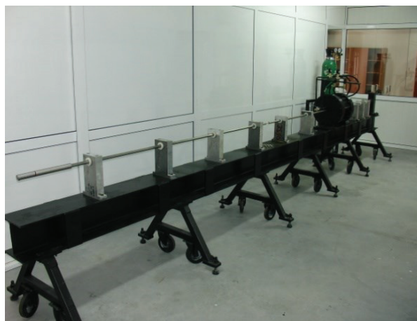
Figure 4.2. Split Hopkinson Tension Bar used in high strain rate tests.
