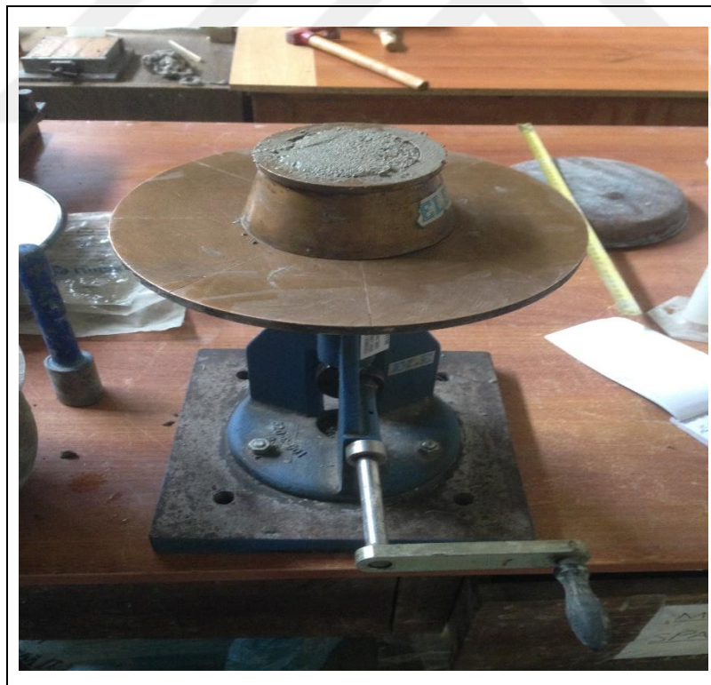
Figure 3.2. Flow table molding
