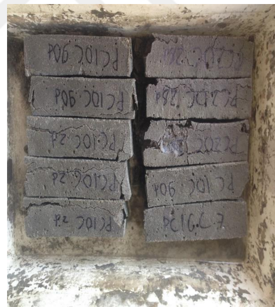
Figure 3.19. Spalled and decayed samples
