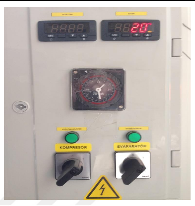
Figure 3.6. Curing cabinet temperature adjustment
