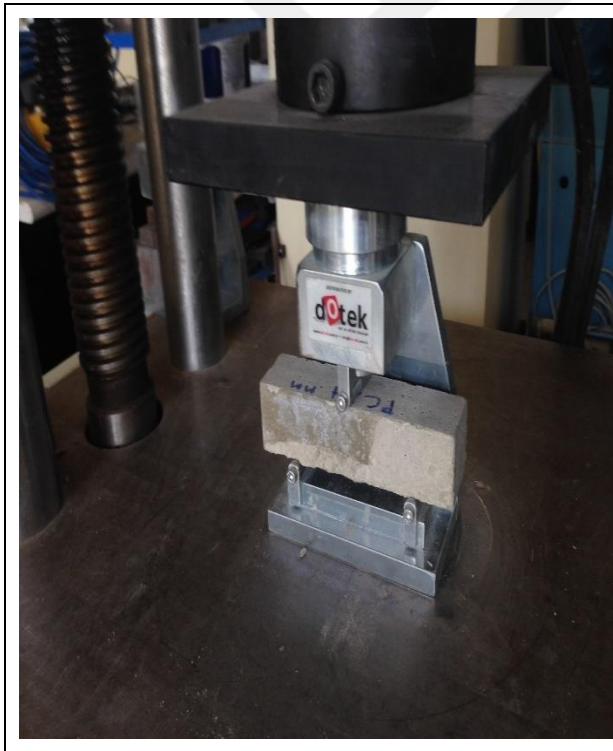
Figure 3.9. Flexural strength test
