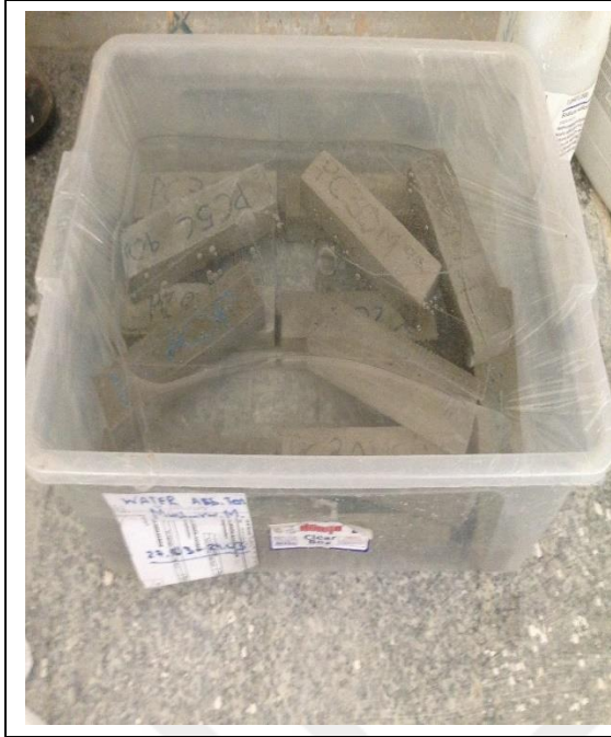
Figure 3.12. Saturation of samples for 72h
