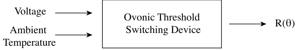
Figure 3.11: For OTS device, the control parameters are ambient temperature and applied voltage.
