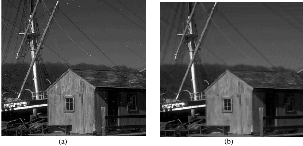
Fig. 4.28 (a) Noisy House image with a low-level noise density of 0.001 (salt and pepper noise), (b) The corresponding reconstructed House image using circular wavelet de-noising scheme; Correlation = 0.9774 and PSNR = 29.9080 dB.
