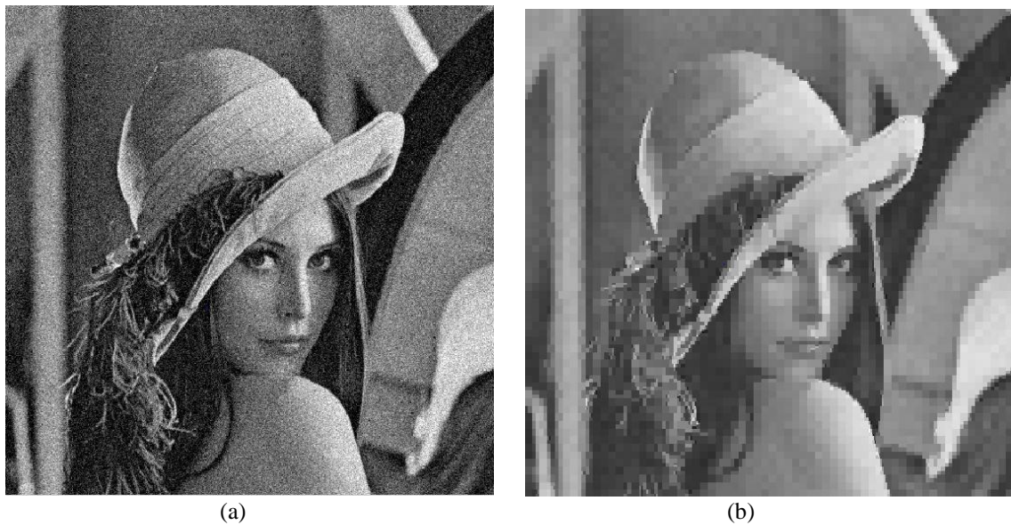
Fig. 4.38 (a) Noisy Lena image with mid-level Gaussian noise; variance = 0.01 & mean = 0, (b) The corresponding reconstructed Lena image using conventional wavelet de-noising by thresholding; Correlation = 0.9636 and PSNR = 25.1233 dB.
