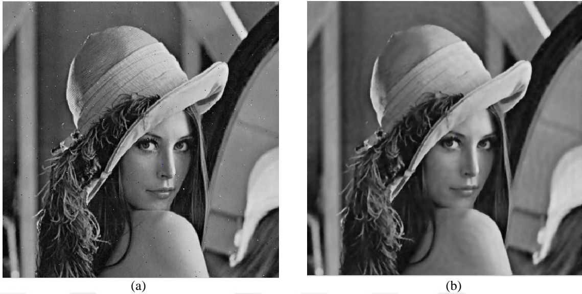
Fig. 4.22 (a) Noisy Lena image with a low-level noise density of 0.001 (salt and pepper noise), (b) The corresponding reconstructed Lena image using circular wavelet de-noising scheme; Correlation = 0.9932 and PSNR = 32.2770 dB.
