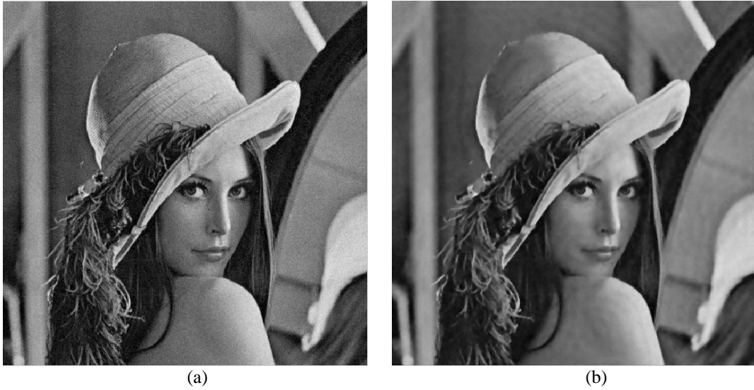
Fig. 4.7 (a) Noisy Lena image with low-level Gaussian noise; variance = 0.001 & mean = 0, (b) The corresponding reconstructed Lena image using circular wavelet de-noising scheme; Correlation = 0.9921 and PSNR = 31.6530 dB.
