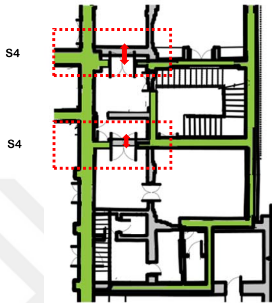
Figure 2.75: Structural Discontinuities in Zone 03 seen by overlapping of Plans Plan at +2.5m Plan at +6.45m
