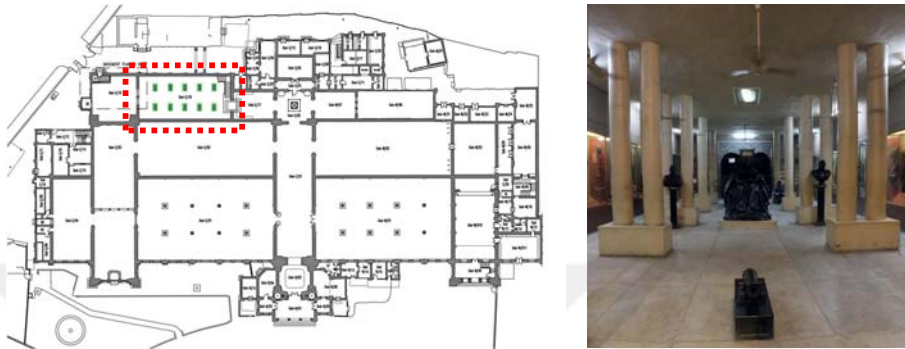
Figure 2.42: Lahore Museum key plan showing location of Reinforced Concrete Columns In Space Gnd-E/18 (left) Looking East rows of RC columns in space Gnd-E/18 (right)
