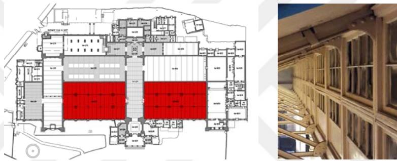
Figure 2.46: Lahore Museum key plans showing locations of saw tooth roof trusses In spaces Gnd-E/01 and Gnd-W/01 (left)
