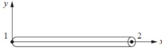
Figure 3.2: Linear element discretization to Line element in FEM
