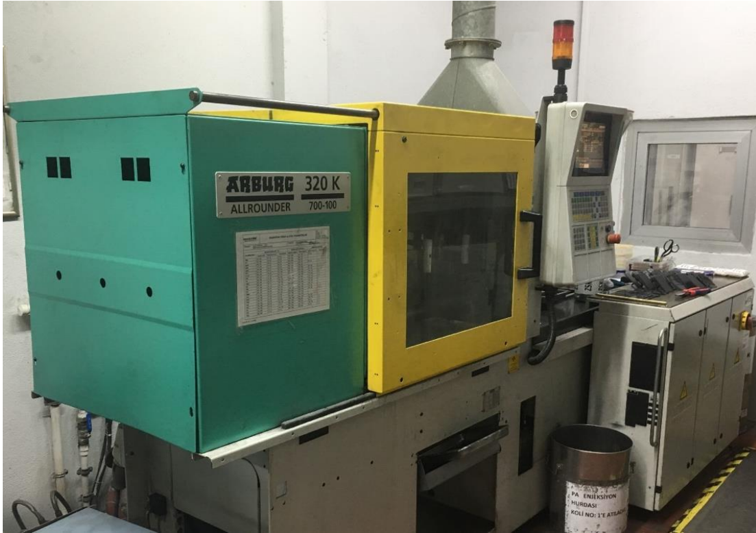
Figure 3.2: Arburg Allrounder 320 K 700-100 injection molding machine.
