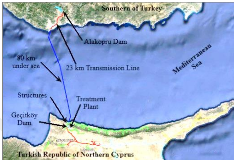
Figure 2.5 TRNC project: constructed pipelines route [54].
