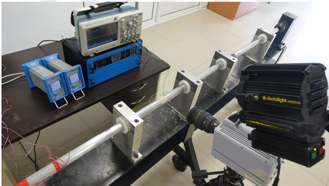
Figure 2.7. Data acquisition and video recording system in the SHPB
