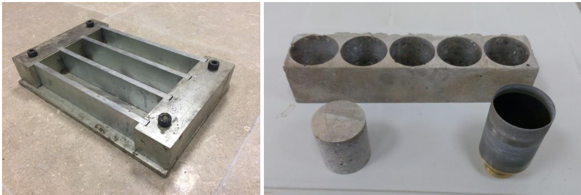
Figure 2.1. Prismatic concrete mold and core-drilled cylindrical test specimen
