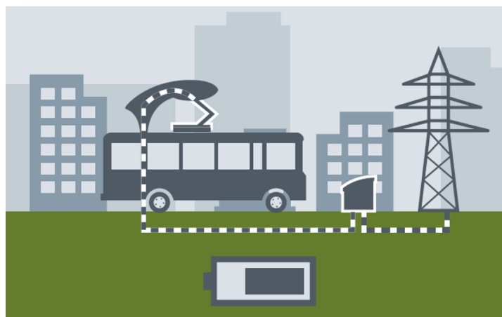
Figure 3.2: Opportunity conductive charging with pantograph.
