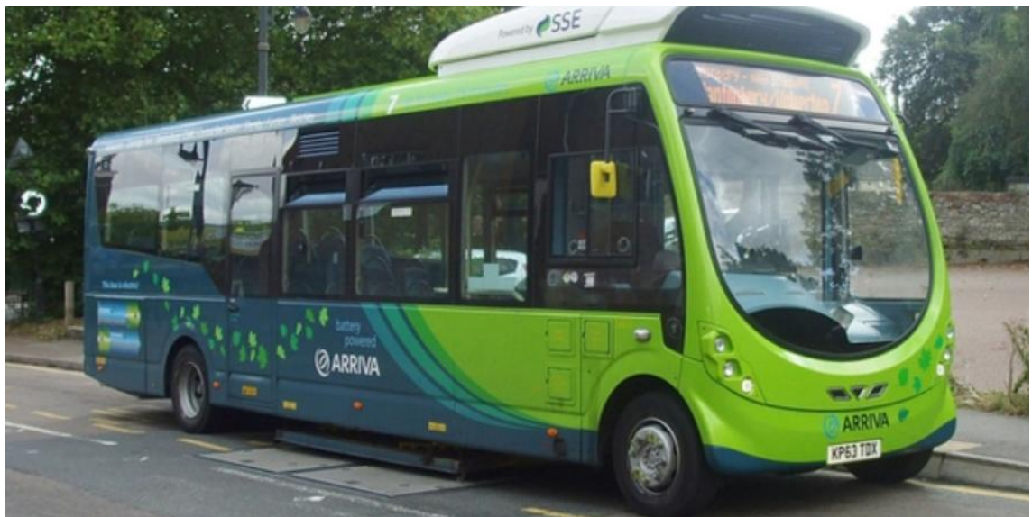
Figure B.4: Outdoor opportunity inductive charging.
