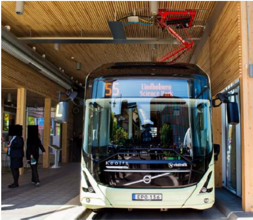
Figure B.3: Indoor opportunity conductive charging with pantograph.
