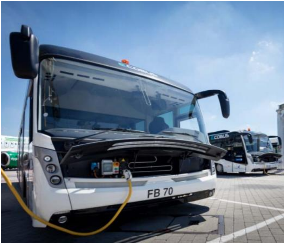
Figure B.1: Plug in charging.
