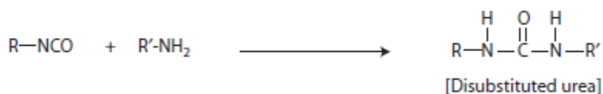
Figure 2.31 : Isocyanate reactions with -NH compounds [16].
