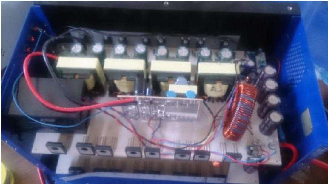
Figure 0.11. Power supply circuit unit
