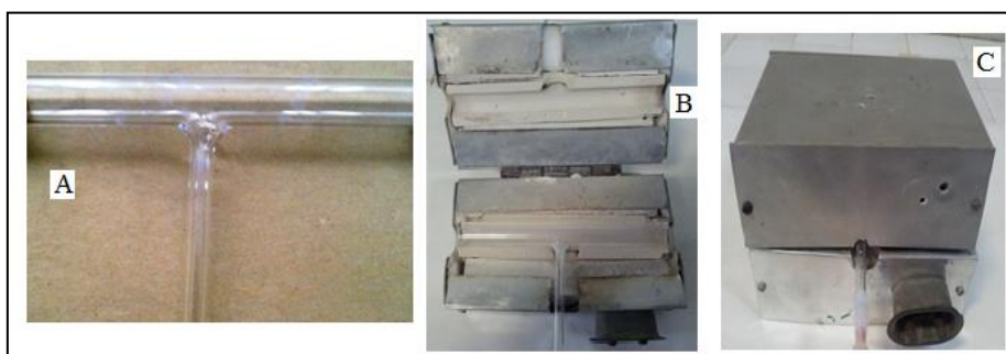
Figure 2.5 The pictures of (A) quartz T-tube, (B) inner area of the electrical furnace with the two semi-cylindrical ceramic parts and (C) the closed electrical furnace
