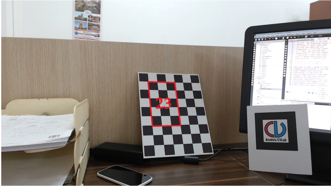
Figure 3.1: False positive example. Marker #23 is detected on the checkerboard pattern. This image is for illustration purpose only, it is not a result of the EDMarkers detection algorithm.
