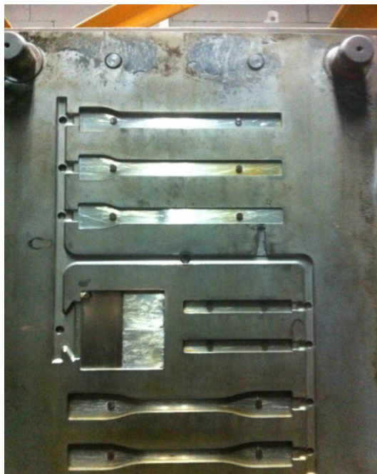
Figure 3.13 : The special mold design of the injection molding machine.
