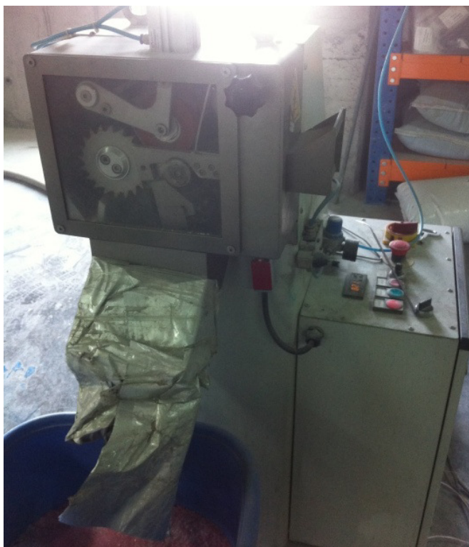
Figure 3.2 : The granulating unit.
