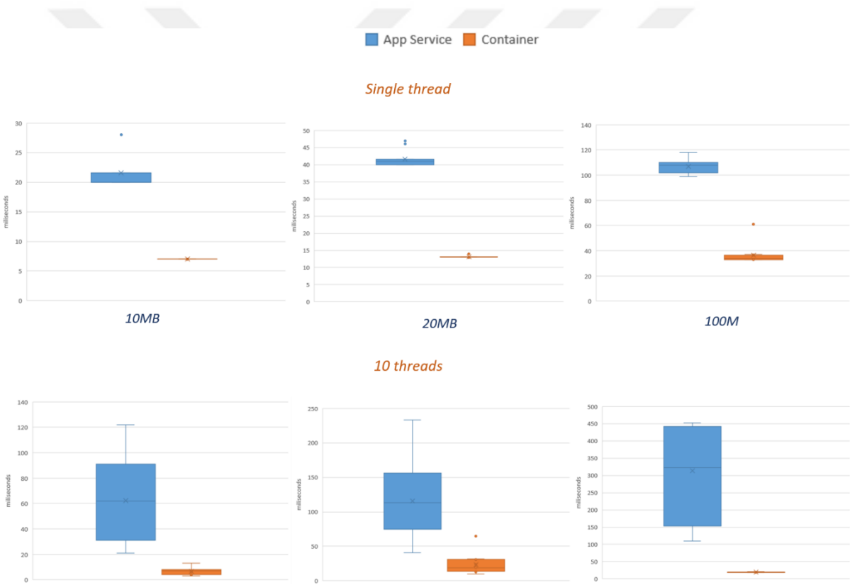
Figure 4.4 Memory read performance comparison between App Service and docker container in Azure
