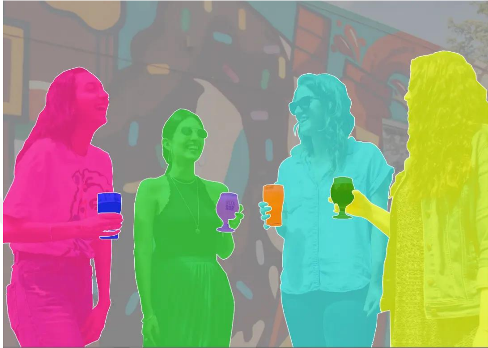
Figure 1.2.1-3 Shows how Panoptic Segmentation works, labels the entire image, credits Super Annotate (2023, August 17)
