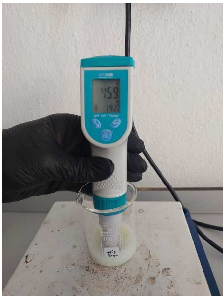
Figure 7. Adjustment of the supernatant pH to 4.6 using HCl for the precipitation of residual casein micelles.
