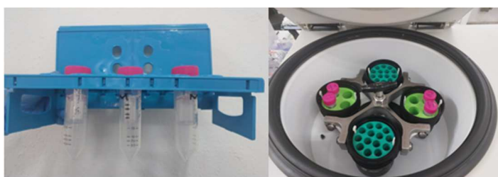
Figure 10. Buffer exchange using Amicon® Ultra-15 centrifugal filter units with a 50 kDa molecular weight cut-off.
