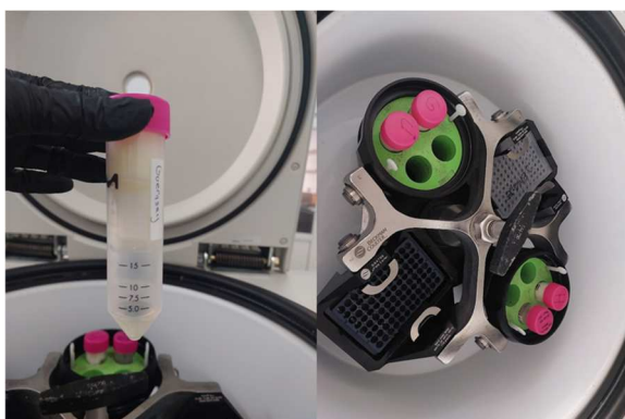
Figure 8. Ultrafiltration of the supernatant obtained after casein precipitation using Amicon centrifugal filter units with a 50 kDa molecular weight cutoff.
