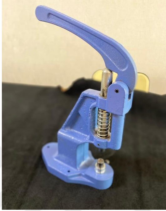
Resim 3.16. Pres Tulumba (Zimba akma Makinesi) Makinesi (İlknur Aytekin arřivi, Ankara, 2024)
