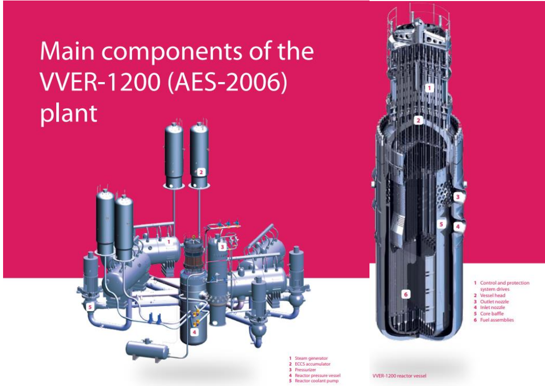
Figure 2.2: Main Components of VVER-1200 plant and Reactor Vessel [31].
