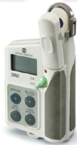
Picture 3.7. Chlorophyllmeter model used in leaf chlorophyll index measurement
