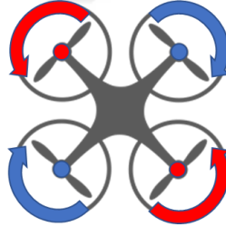
Figure 3.4: Rotors spins in opposite direction
