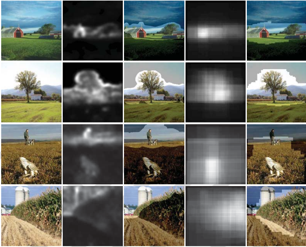
Figure 6.6. Visual attention-driven feature pooling scheme. For a given image a bottom-up saliency map and (b) an object-level saliency map are estimated and then the feature vectors are pooled over the salient regions of the images (depicted as bright areas in the images).
