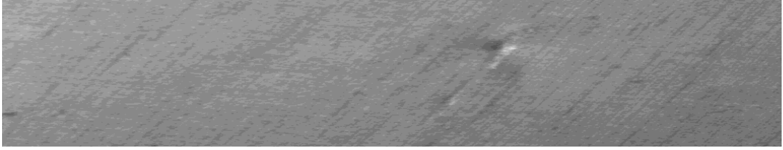
Figure 4.4. Thread defects in the center of the picture
